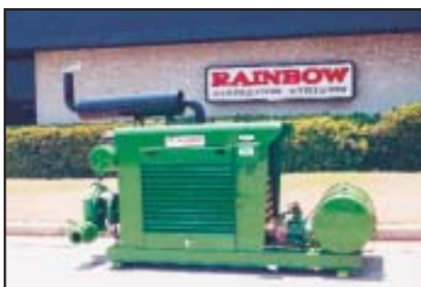
High Pressure Booster Pump
