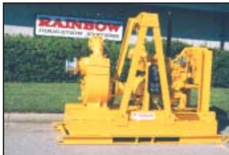
Skid Mount Dewatering Unit
