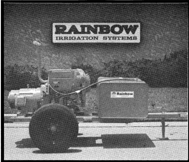
DEUTZ F3L1011 W/ 15KW GENERATOR
